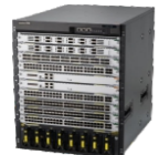
NSS11500-08 - CLOS Architecture - Eight Service Slots
